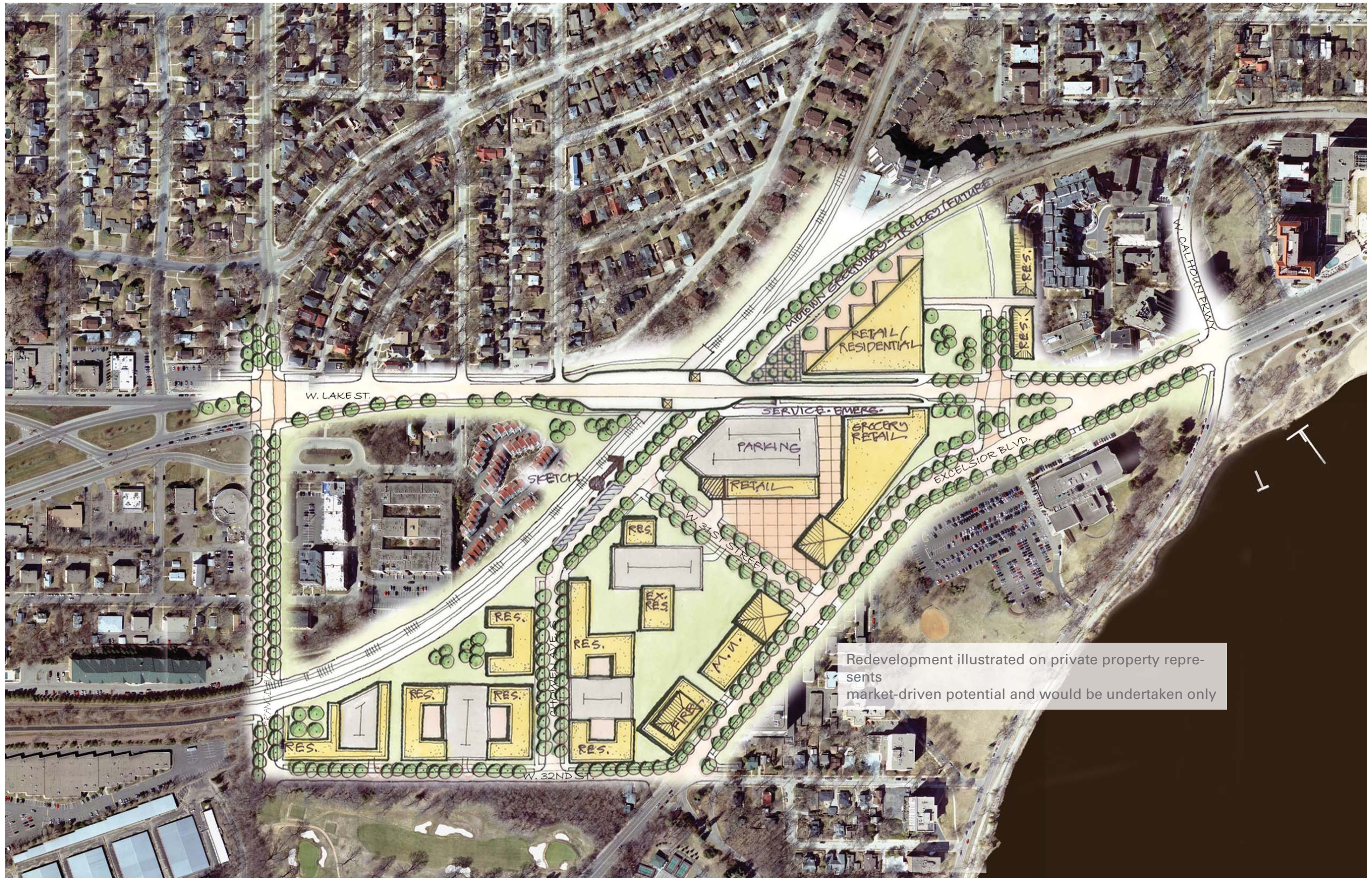
West lake Station: Sample Transit-Oriented District. Increased residential density promotes LRT ridership. Redeveloped retail nodes places buildings against the street and structures parking within the lot in order to create a pedestrian-scale, walking environment.
