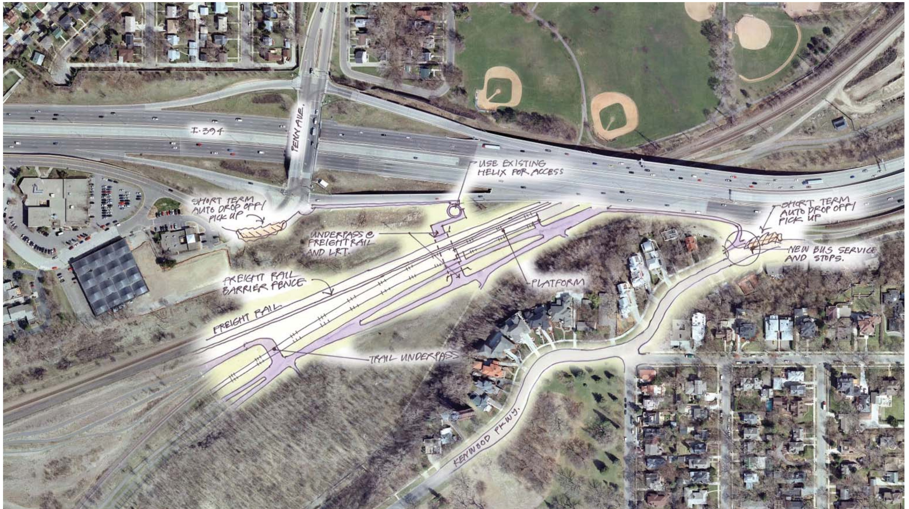
Penn Station: Opening Day Recommendations. Pedestrian access across the freight rail tracks is critical to transit ridership. This option illustrates a pedestrian underpass at the foot of the existing ped/bike helix.
