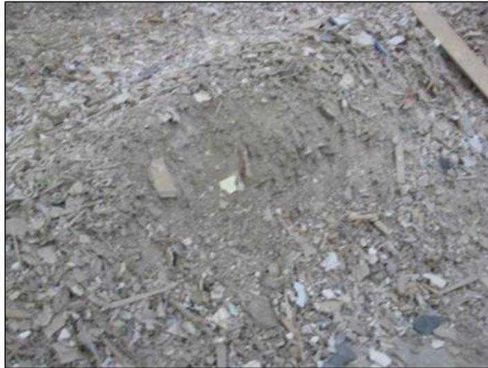
ADC includes dirt, wall board, masonry, small pieces of cardboard and paper, rocks, and plastic all in smaller pieces (either 2 inch or 3 inch minus). ADC generally has little to no BTU energy value as most of it is inert aggregate-like material. It can be economically sorted via mechanical screens from mixed C&D, but it has few other uses other than landfill ADC.
