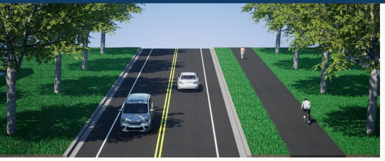
Original recommended design: **51 ft** from edge of curb to edge of path
