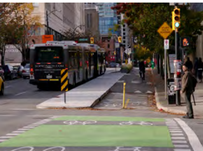
Dunsmuir Street, Vancouver, Canada: Two-way cycletrack alongside a bus route and one-way auto traffic. Buses load in lane from a median located between the cycletrack and the bus lane.
