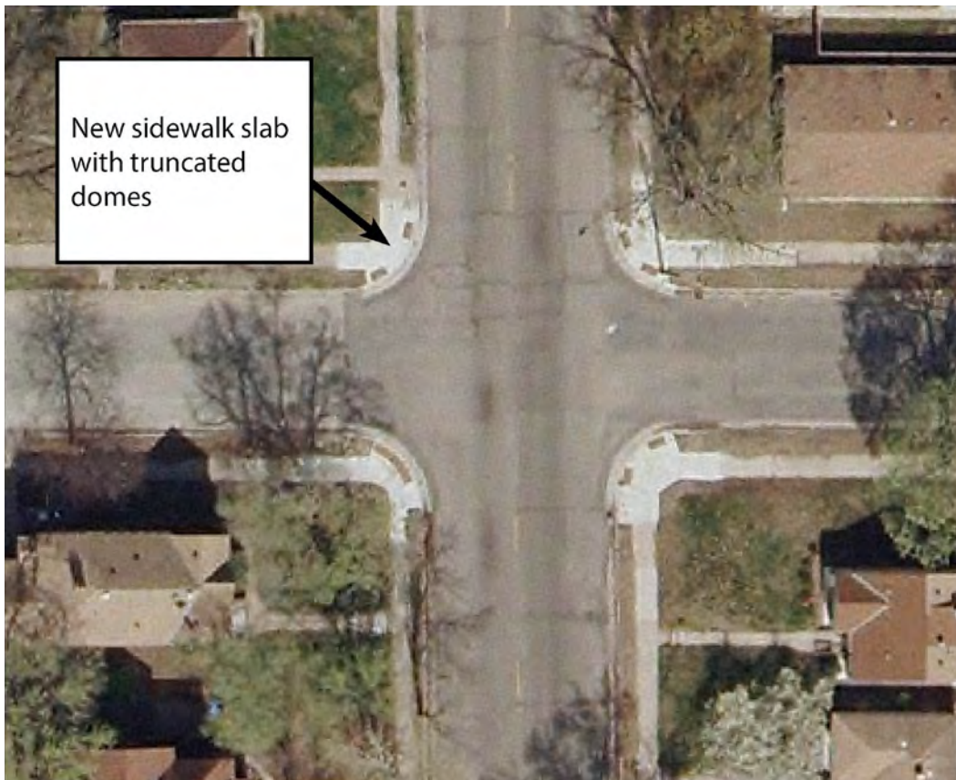
FIGURE 6-2: TYPICAL INTERSECTION UPGRADE
