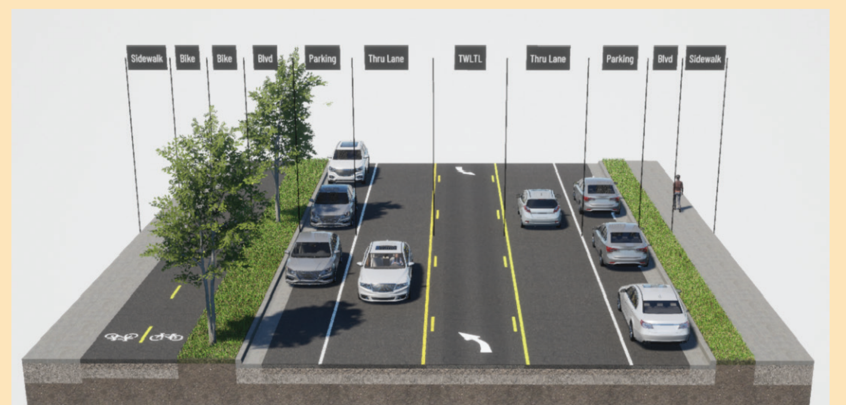
Southern section (upper portion): two-way off-street bikeway with two-way left turn lane (two lanes of parking)
