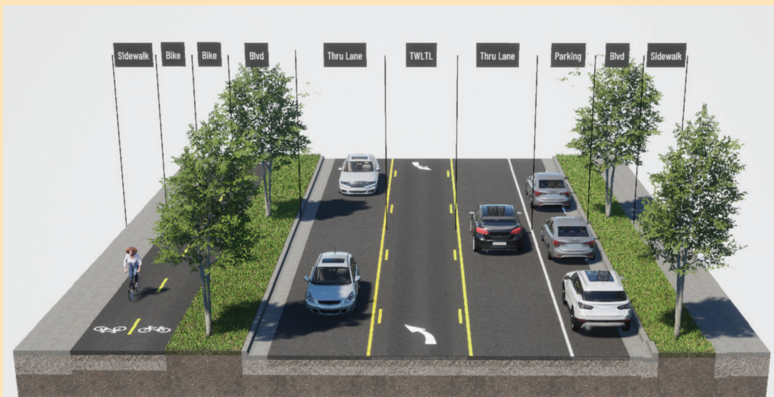
Southern section (lower portion): two-way off-street bikeway with two-way left turn lane (one lane of parking)
