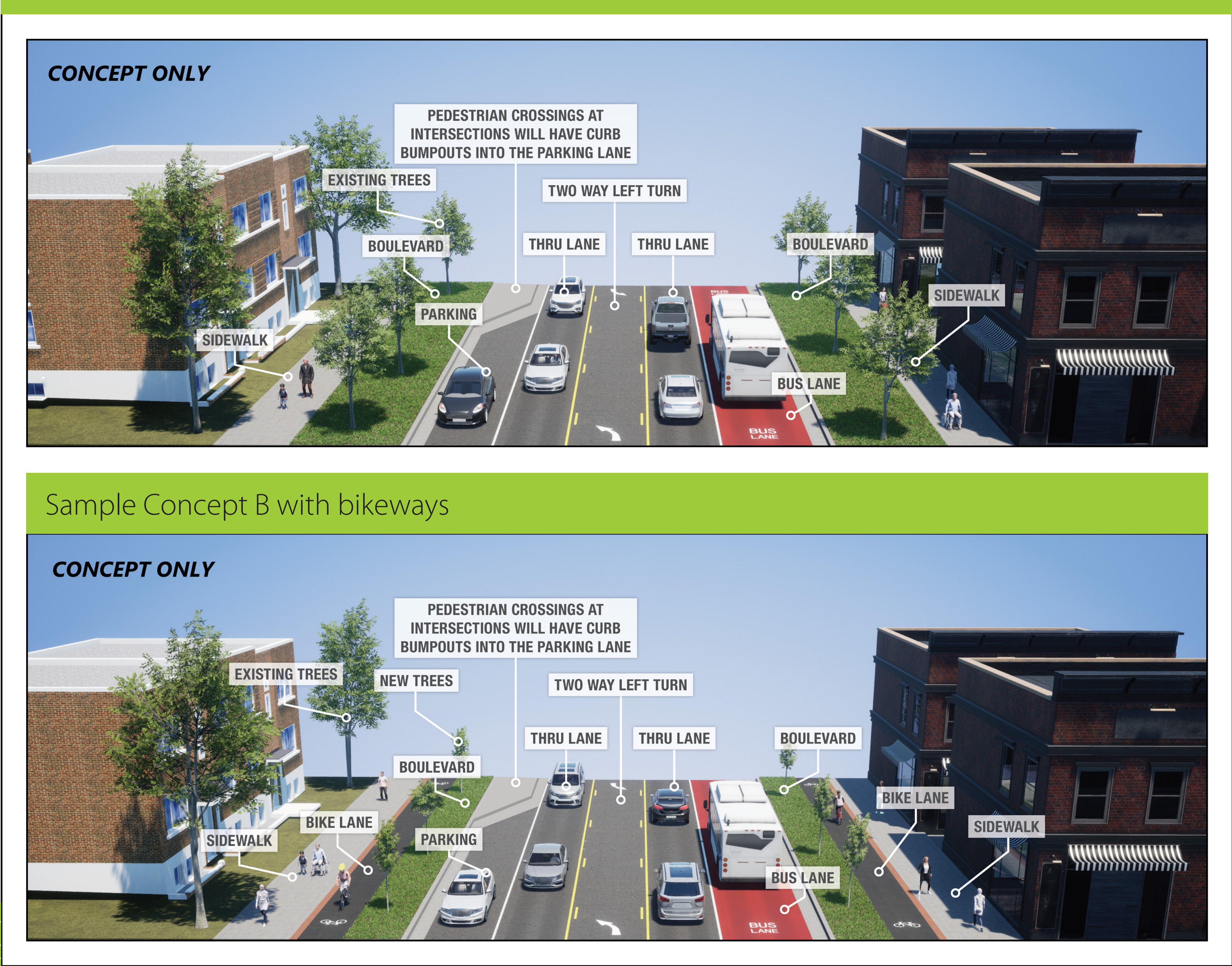
Bikeways for consideration between Summit Avenue and 28th Street. These section concepts do not reflect the final options for the corridor layout.
