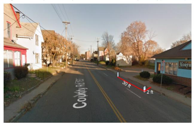
Figure B6: How to paint Broadway St NE four lane road without bicycle facility (Not to Scale)
