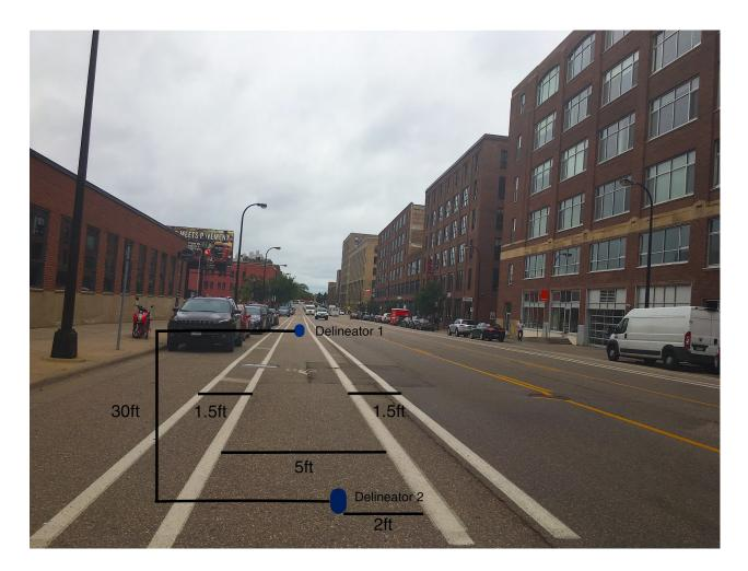
Figure B1: How to Delineate Washington Ave Buffered Bike Lane (Not to Scale)
