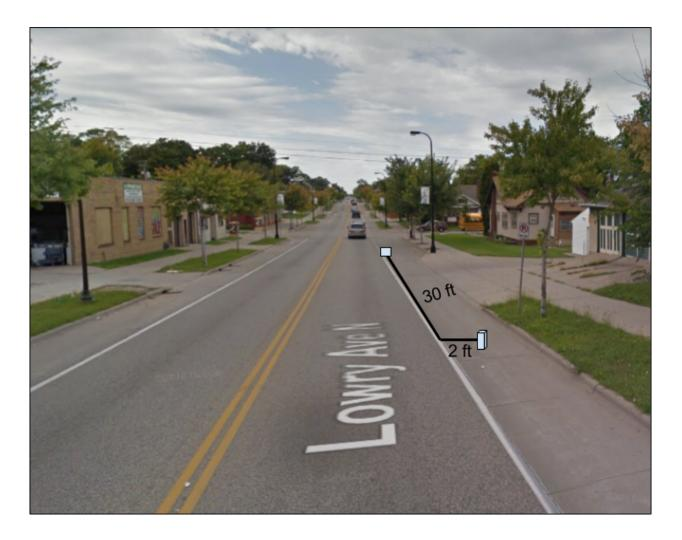
Figure B3: How to Delineate N Lowry Ave- Bike Lane (Not to Scale)
