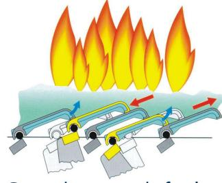
Grate bars push fuel up & forward as it burns. Air injected above & below grates.
